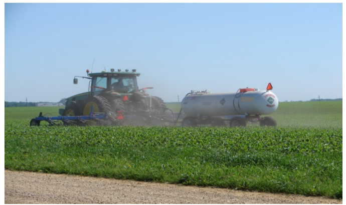
Figure 2. Anhydrous ammonia sidedress application to V5 corn.
