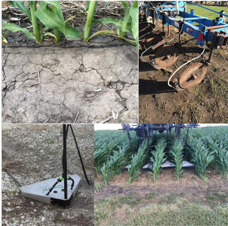
Figure 3. The 360 Y-Drop® unit applies nitrogen (N) to the base of the plants (top left), rolling coultter applicator applies the N behind the coultter as it cuts through the soil (top right), 360 Y-Drop® unit (bottom left), and 360 Y-Drop® applicator (bottom right).
